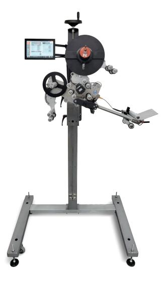
The NITA 100% servo driven stand-alone labeling head is made for applying labels to whatever, whenever. Geek out on up to 3200 inches per minute of super accurate label application.
